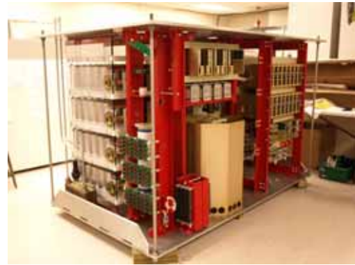
Figure 4. The ILC Modulator is a compact unit, for immersion in a 7' x 5.5' oil tank, with controls on top and coax cable pulse output.
