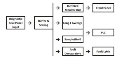
Figure 1. Block Diagram of one analog channel.
