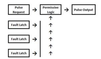
Figure 2. Block Diagram of fault logic permitting pulse pass-thru.
